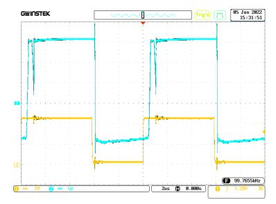
Figure 14. The voltage waveforms of inductors L<sub>2</sub>
