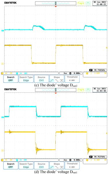
Figure 11. The diodes' voltage  $D_{forward}$ ,  $D_{flyback}$ ,  $D_{out2}$  and  $D_{out1}$
