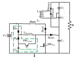
Figure 1. Proposed converter circuit
