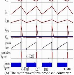
Figure 3. The waveform corresponds to the main converter drive switch and the snubber circuit switch
