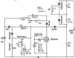
Figure 4. The proposed converter in PISPIS s/w environment
