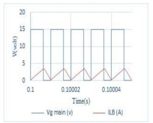
Figure 6. Non coupled inductor-branch current (L<sub>B</sub>)
