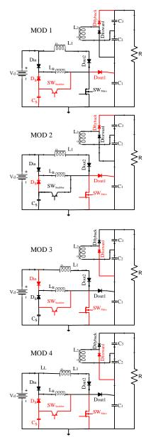
Figure 2. The modes of the proposed converter
