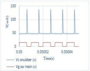
Figure 7. The main gate switch voltage and the capacitor SNUBBER voltage
