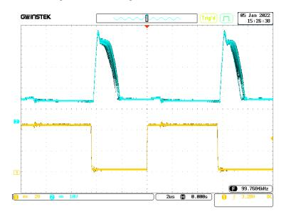
Figure 15. The Snubber capacitor voltage and the gate voltage of main switch
