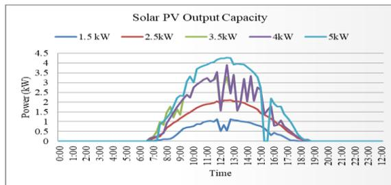
Figure 4. Solar inverter output variations
