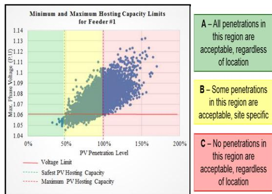
Figure 8. Maximum phase voltage variation against solar penetration level
