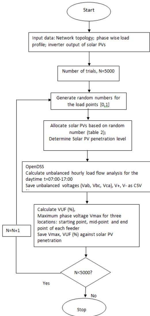
Figure 2. Flowchart for determination of voltage unbalances using Monte Carlo simulation
