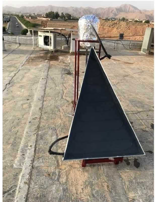
Figure 1. Photo of the triangular flat plate collector
