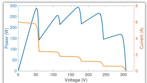
Figure 4. PV characteristic curves in the case of non-uniform shading condition.
