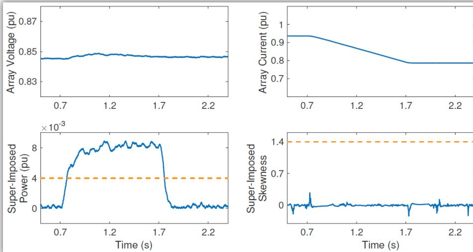
Figure 9. Performance of the developed algorithm in the case of a non-severe partial shading condition.
