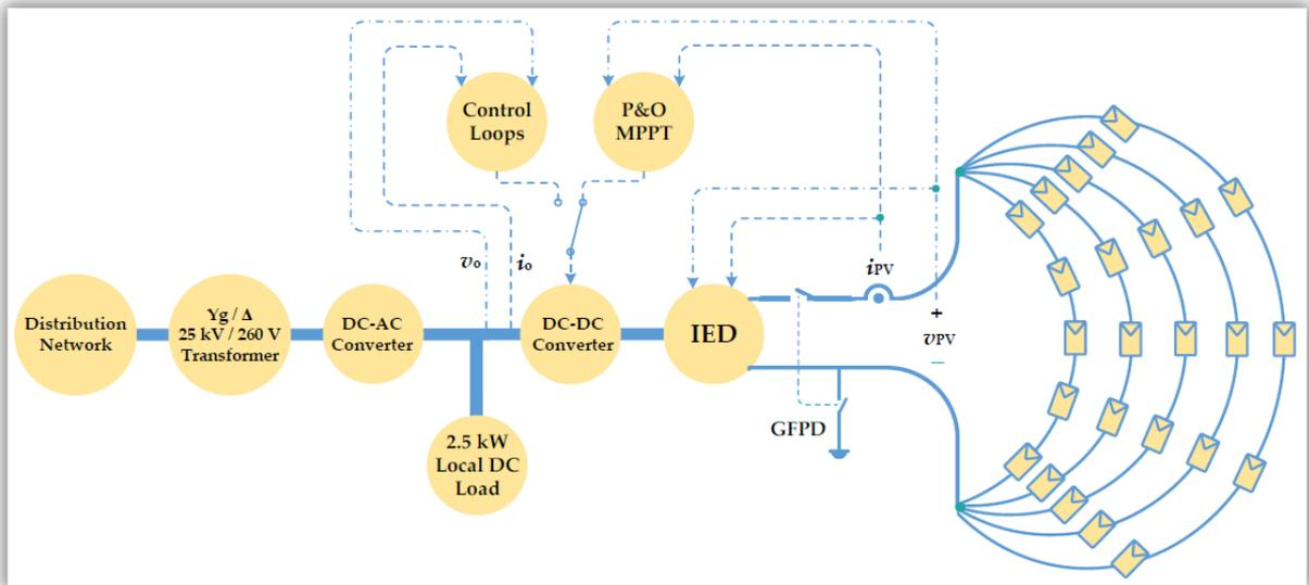
Figure 7. Layout of the study grid-connected PV array.
