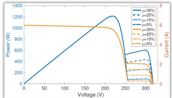
Figure 3. PV characteristic curves under various shading strengths.
