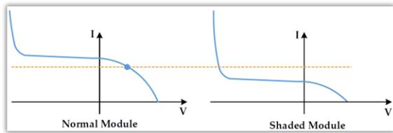
Figure 5. *I-V* characteristic curves of series normal and shaded modules.
