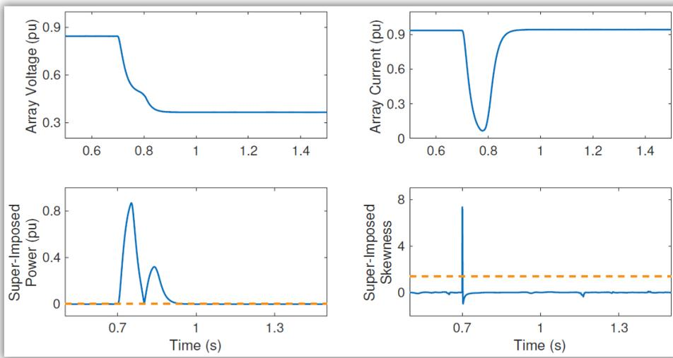
Figure 10. Performance of the developed algorithm in the case of a severe short-circuit condition.
