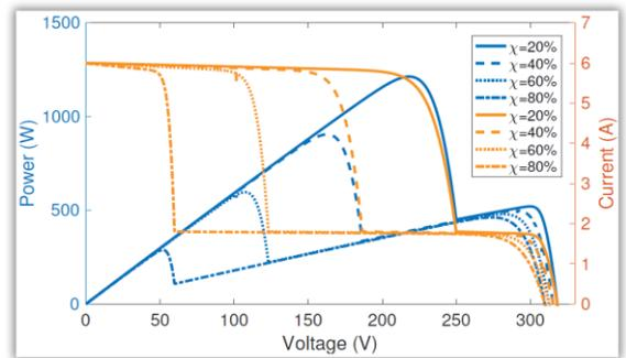
Figure 2. PV characteristic curves under various shading rates.
