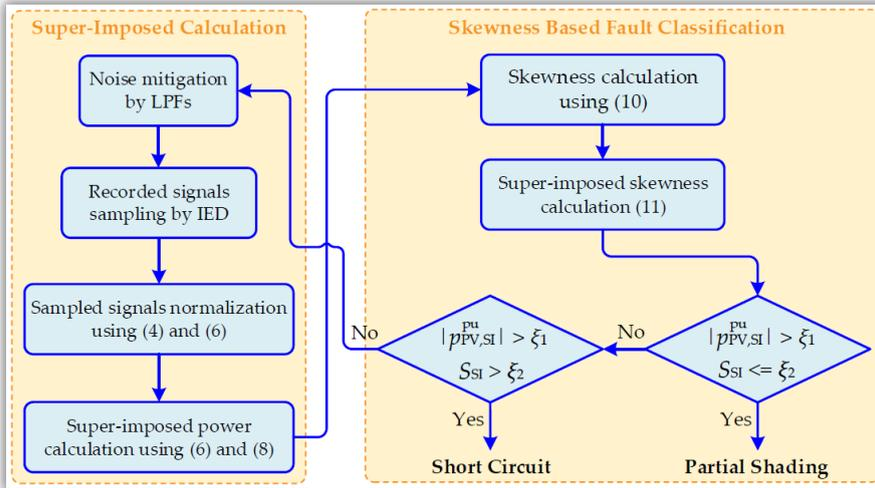
Figure 6. Flowchart of the developed partial shading condition detection algorithm.
