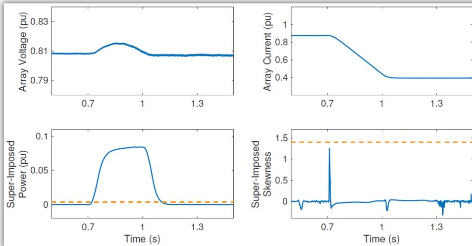
Figure 12. Performance of the developed algorithm in the case of a severe partial shading condition considering parameter uncertainty.
