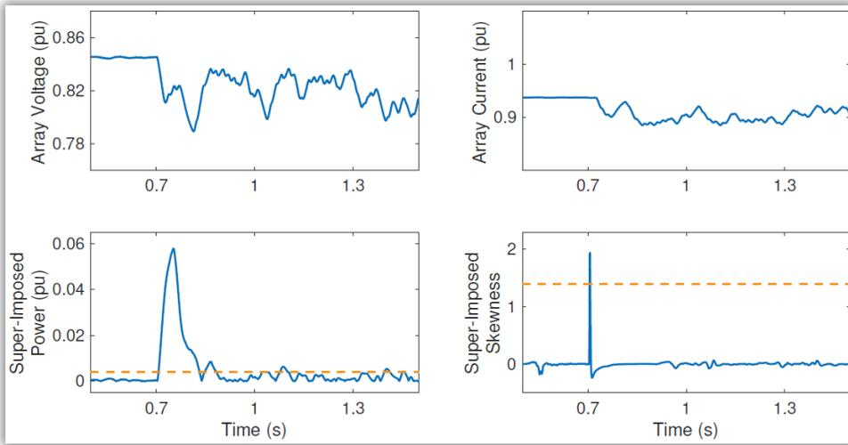
Figure 11. Performance of the developed algorithm in the case of a non-severe fault condition.
