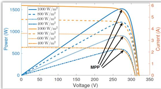
Figure 1. PV characteristic curves under uniform solar irradiation.
