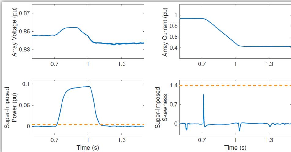
Figure 8. Performance of the developed algorithm in the case of a severe partial shading condition.
