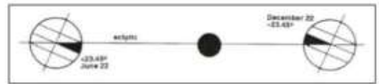
Figure 3: 2D section of earth's orbit, showing the two extreme declination angles, Source: [29]
