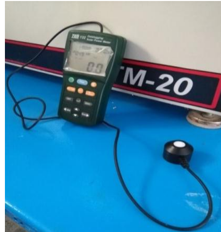
Figure 7. The solar power meter datasheet model TES-132
