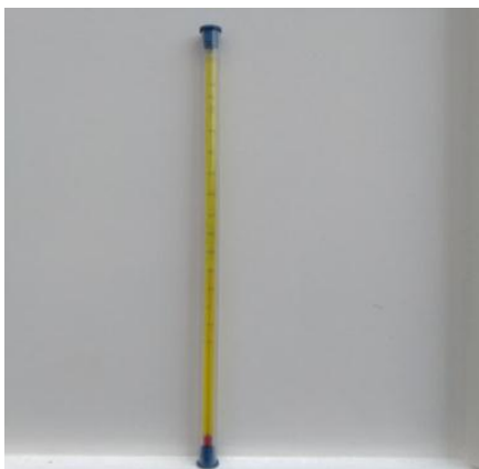
Figure 6. Mercury Thermometer for measuring water temperature
