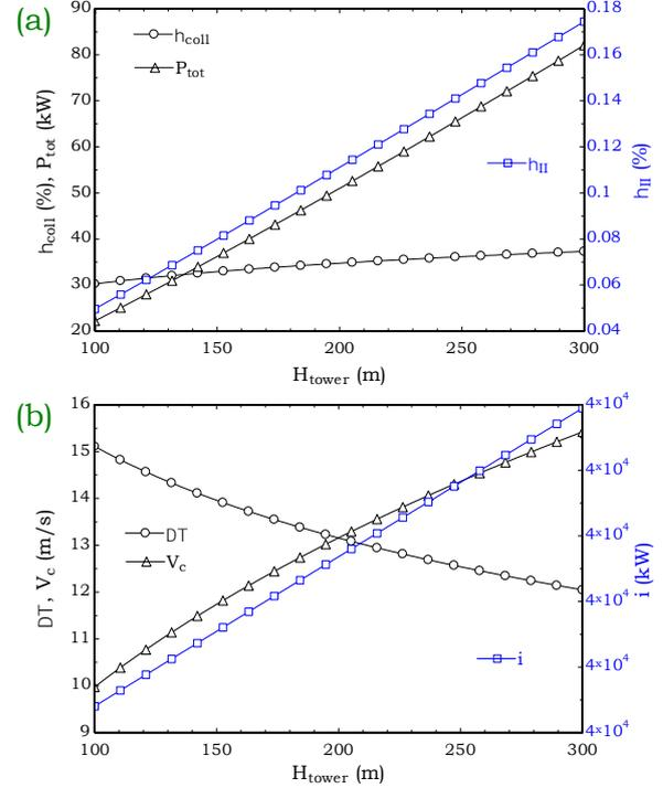
Figure 5. Effect of tower height on SCPP performance
