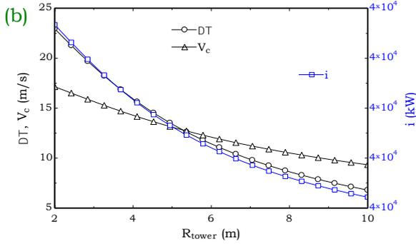
Figure 3. Effect of tower radius on the SCPP performance
