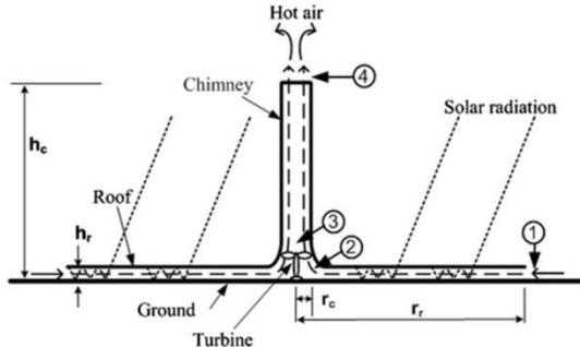
Figure 1. Schematic of a conventional SCPP
