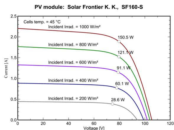
Figure 1. current-voltage curve of the module for various radiations.
