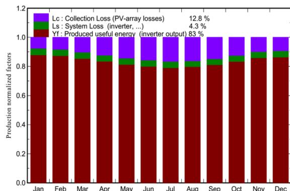
Figure 3 . Loss factors using PVsyst software
