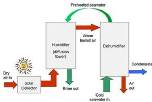
Figure 6. A simple humidification–dehumidification (HDH) process
