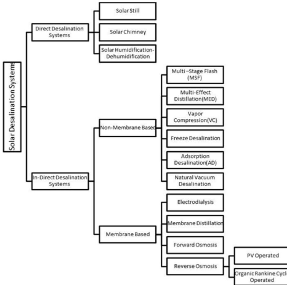
Figure 1. Classification of solar desalination systems
