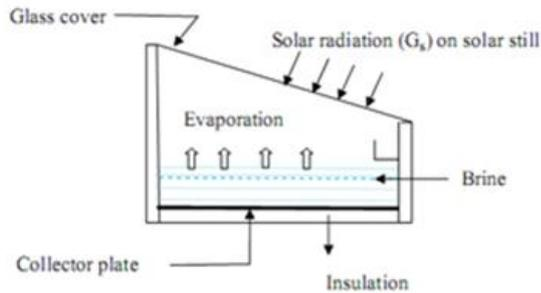
Figure 2. The schematic view of a single effect single slope basin type conventional passive solar still
