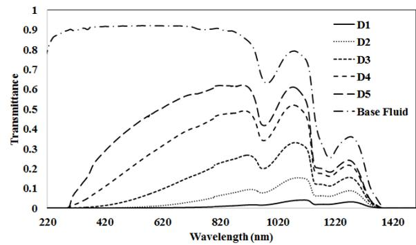
Figure 4. Transmittance spectra of nanodiamond nanofluid samples
