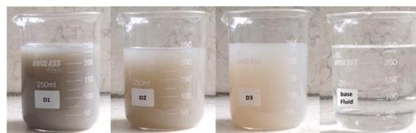
Figure 2. Three different weight fractions of diamond nanofluids
