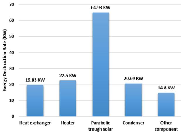
Figure 2. Exergy destruction rates for main components of system
