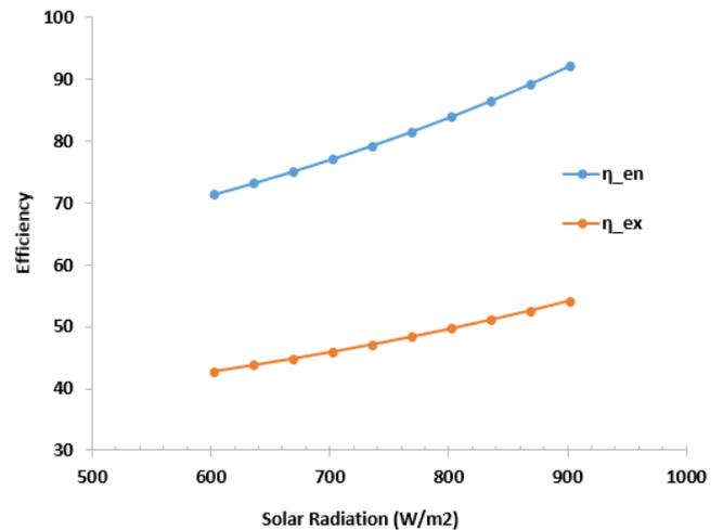
Figure 4. Effect of solar radiation on system performance
