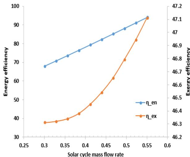
Figure 6. Effect of solar cycle mass flow ratio on system performance
