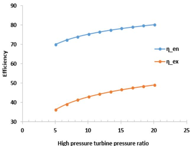
Figure 5. Effect of high-pressure turbine pressure ratio on system performance
