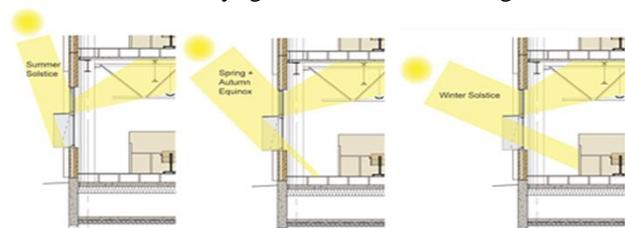
Figure 1. Daylight control [5]
