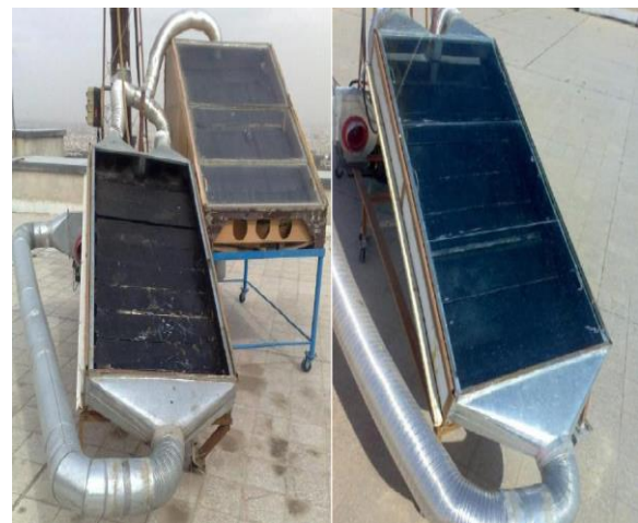
Figure 1. The presentation of the solar dryer and thermal energy storage containers
