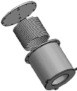
Figure 2: designed cavity receiver
