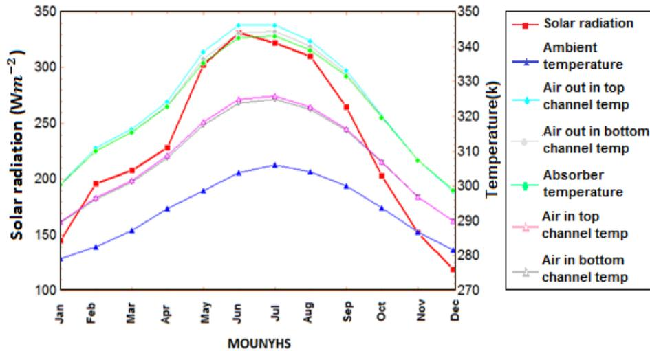
Figure 4. Monthly variation of solar radiation and temperature of solar air heater components.
