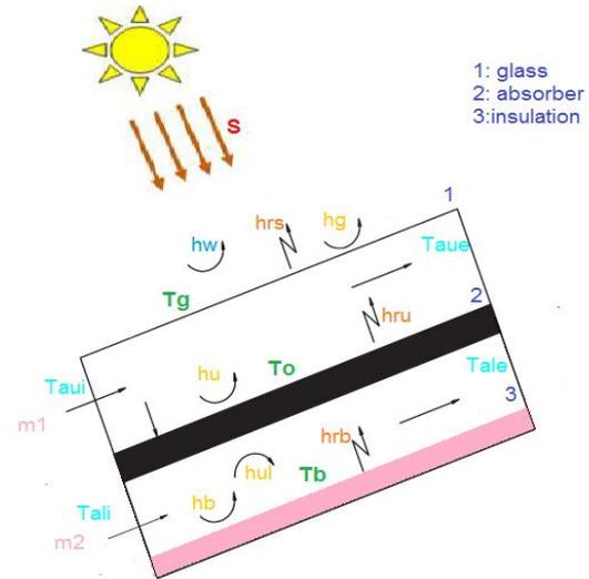
Figure 1. Schematic of solar air heater with heat transfer coefficients.
