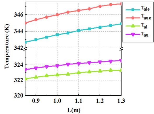
Figure 2. Effect of inlet length variation of collector on value of top and bottom channel temperatures.
