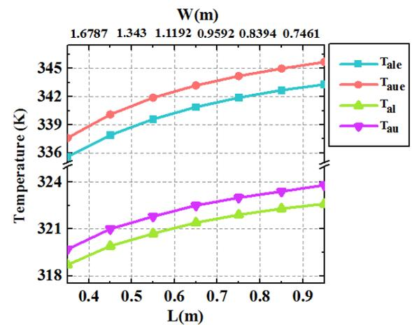
Figure 3. Effect of length variation and inlet width variation of collector on value of top and bottom channel temperatures with fixed area ( $A = 0.6715 \text{ m}^2$ ).
