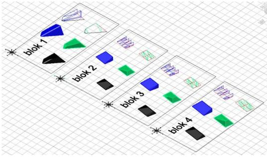
Figure 6: Solar envelope generation for the analyse of the current case.
