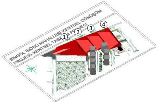
Figure 7: The obtained solar envelopes for the current case and their superposition with existing buildings.
