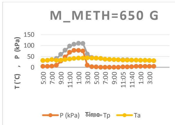
**Fig. 4.** The variation of collector temperature, pressure and ambient temperatures (23 May 2016)
