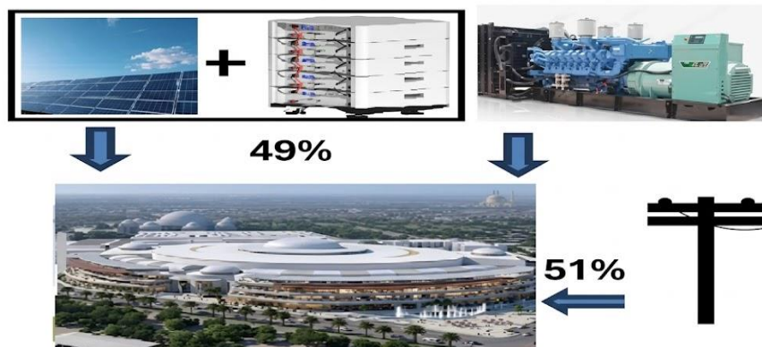
Figure 12. The hybrid -grid power system components
