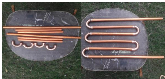
Figure 5. Mechanism of manufacturing the coil inside the shell for the parts
