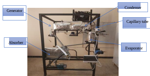
Figure 7. Absorption system cycle
