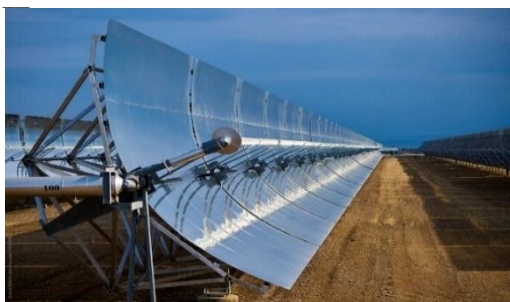
Fig .1 photograph of parabolic trough collector (concentrator) [11]
