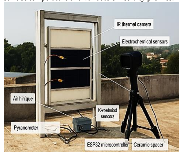
Figure 3. Rooftop test setup
