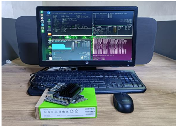
Figure 6. Embedded implementation of the proposed method using Jetson Nano
