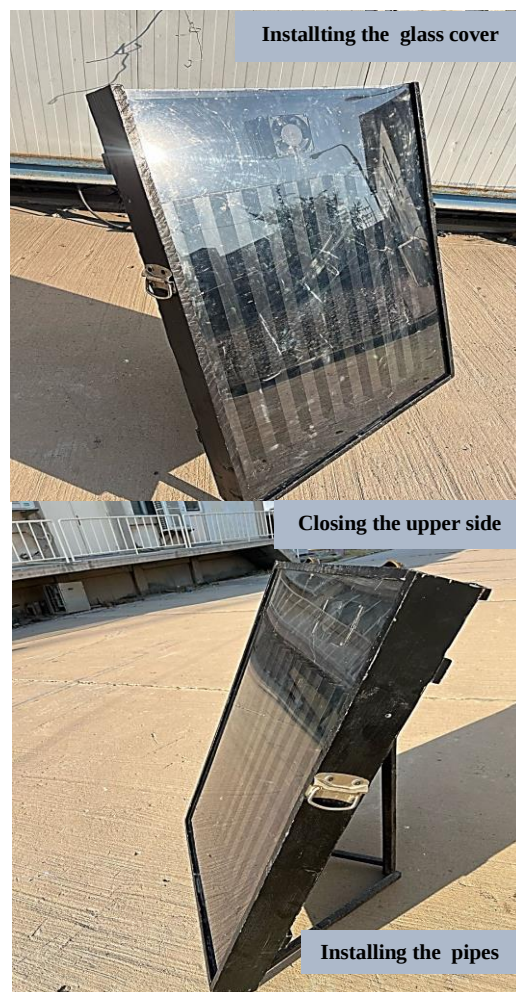
Fig. 4B. Manufacturing of the SAH.
