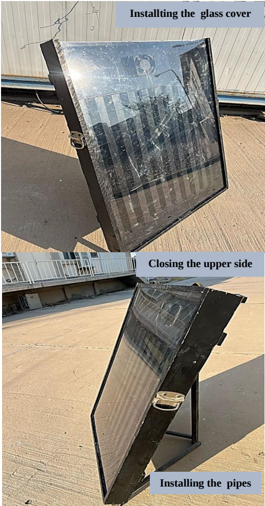
Fig. 4B. Manufacturing of the SAH.
