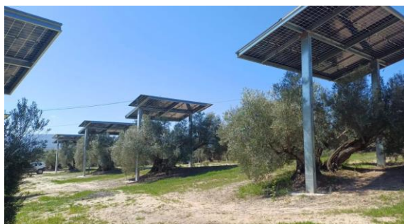
Figure 4. Overhead Olivoltaic experimental setup in Jaén, Spain
