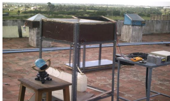
Fig. 36 Solar box cooker with nanocomposite material [103]
