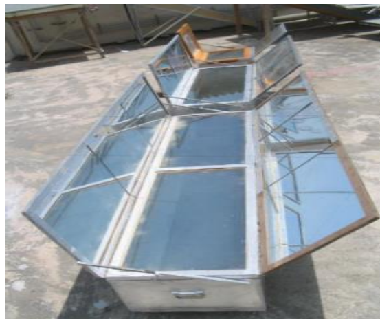
Fig. 17 Solar box cooker with three different aspect ratios with two booster mirrors [61]
