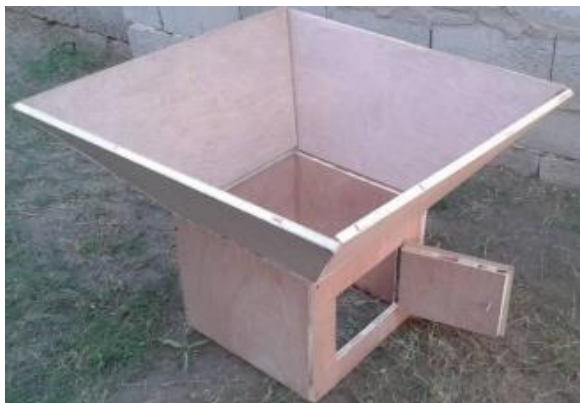
Fig. 18 Solar box cooker with four reflectors [57] Ademe et al. , [83] fabricated a solar cooker comprising a 50 mm single-walled cardboard box, as shown in Fig. 19. The inward box was developed utilising an iron sheet 1.5 mm thick. The space between the outer and inner tubes was filled with 50 mm-thick sawdust as an insulator. Three adjustable reflectors were mounted to reflect the radiation onto the absorber plate's base and sides. The reflectors' inward pieces were fabricated from a 1.5 mm-thick iron sheet. The authors concluded that three reflectors with a double-glazing solar cooker with 1.43 kg of
