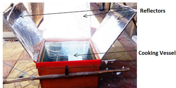
Fig. 19 Box-type cooker with three reflectors [83] 4.4 Comparison
