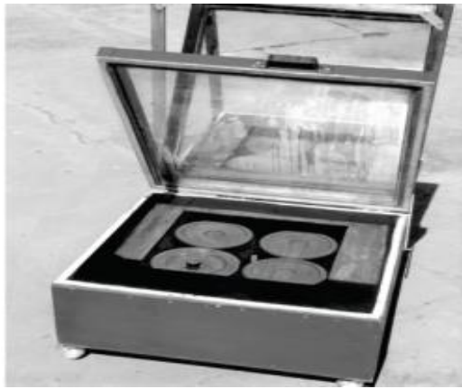
Fig. 28 A solar cooker with a double-glazed, high-insulation box and a reflector [93]
