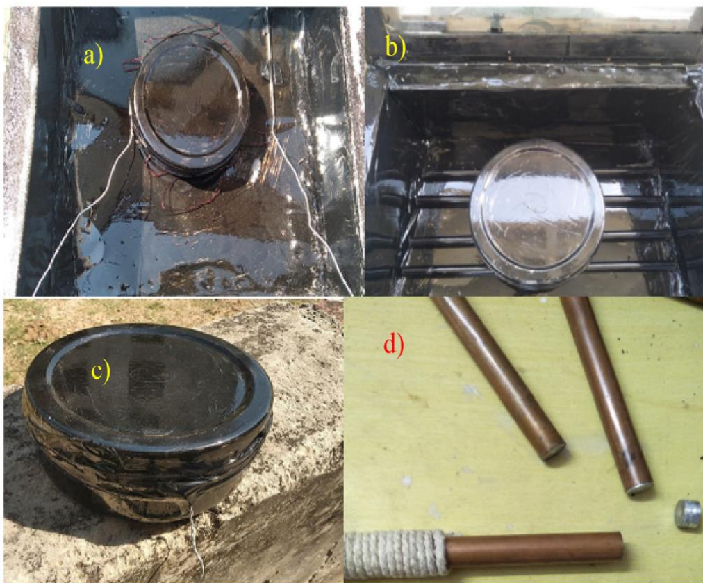
Fig. 38 Solar box cooker with flexible solar collector tubes [105]
