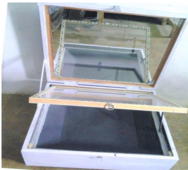
Fig. 23 A white water glass in a double-glazing cover of a new box-type cooker [88]
