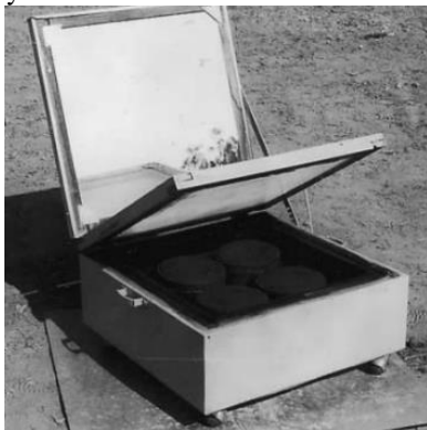
Fig. 8 Solar box cooker with four cooking vessels [71]
