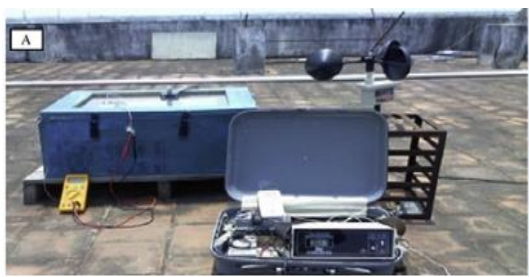
Fig. 39 Solar box cooker with PCM and Nanoparticles [106]
