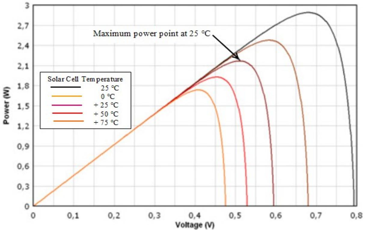
Figure 3. b) Influence of PV panel temperature on output parameters such as voltage [39].
