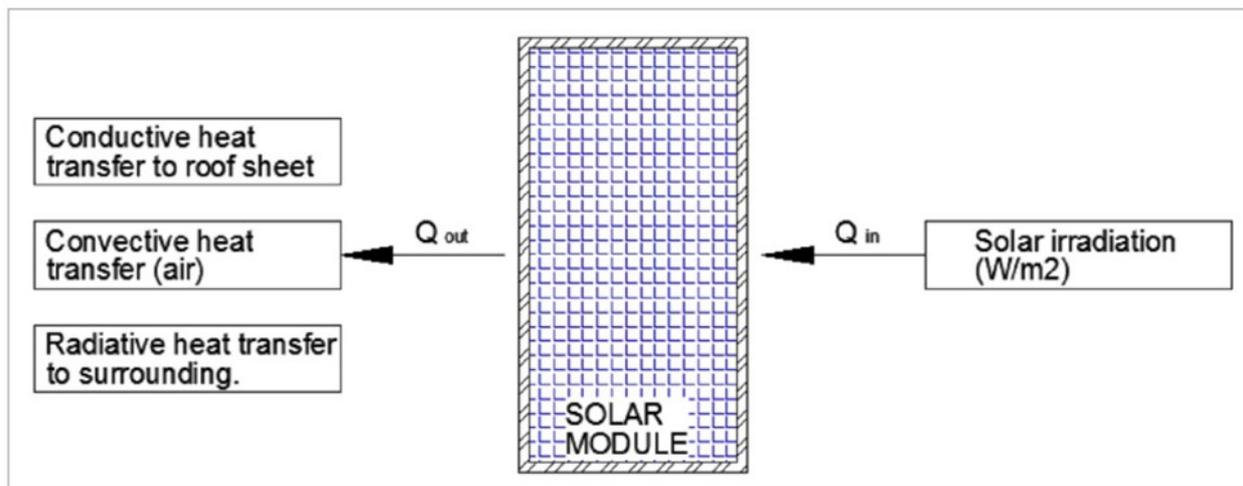
Figure 2. Heat balance of the solar module [36]
