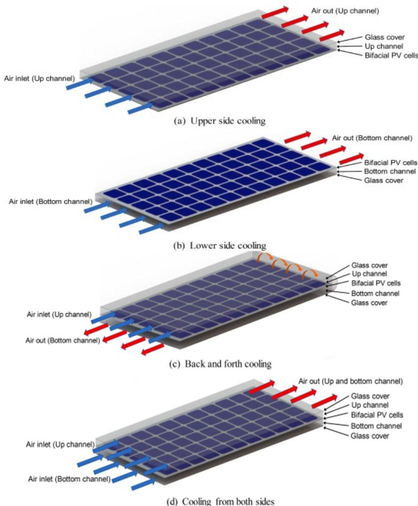
Figure 6. Various cooling techniques have been applied to BPV/T modules [47].
