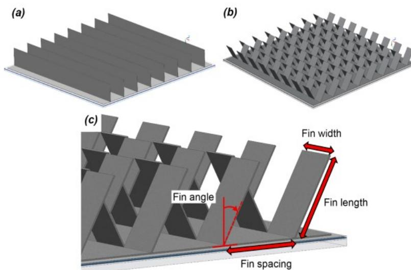
Figure 7. PV cooling system, (a) conventional heat sink, (b) proposed heat sink, and (c) fin parameters [48]
