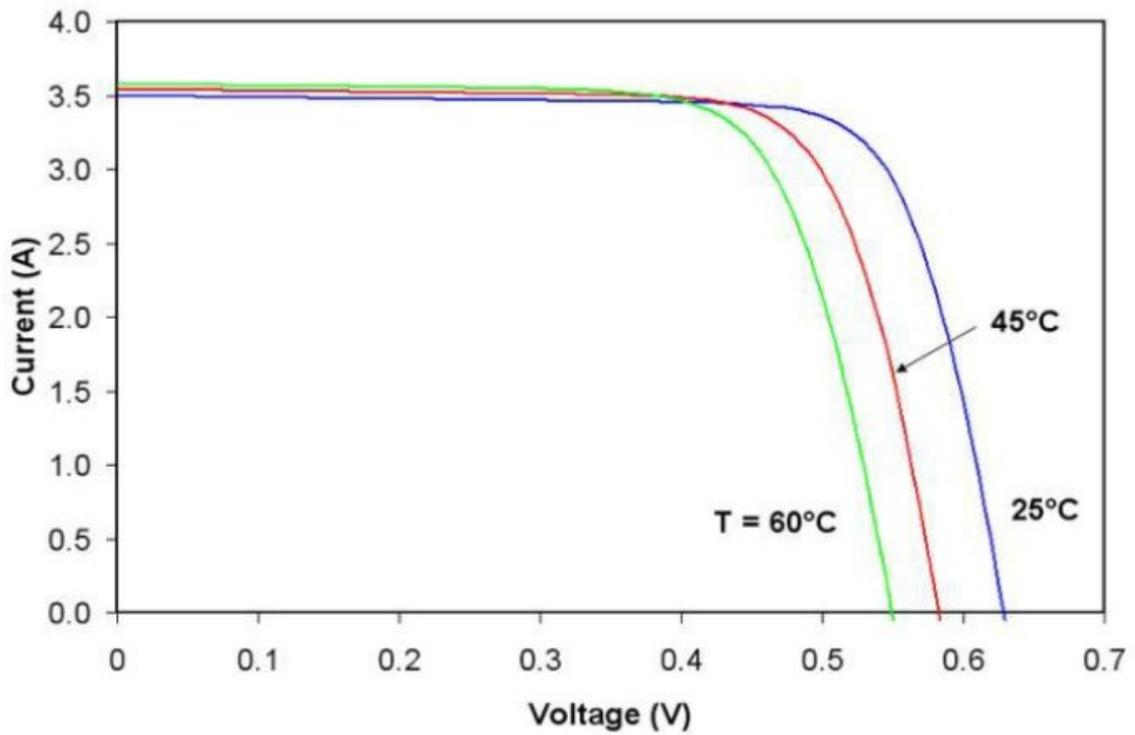
Figure 3. a) Influence of PV panel temperature on current output parameters [39]
