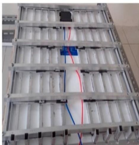
Figure 10. Floating PV experimental configuration of (a) thermosiphon-floating PV system and (b) bottom view of solar module attached to heat-absorber pipes [67].
