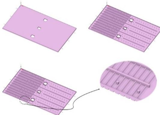
Figure 9. Cooling box design [66]
