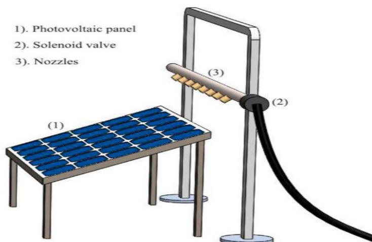
Figure 11. PV panel schematic view with spray-cooling system [71]
