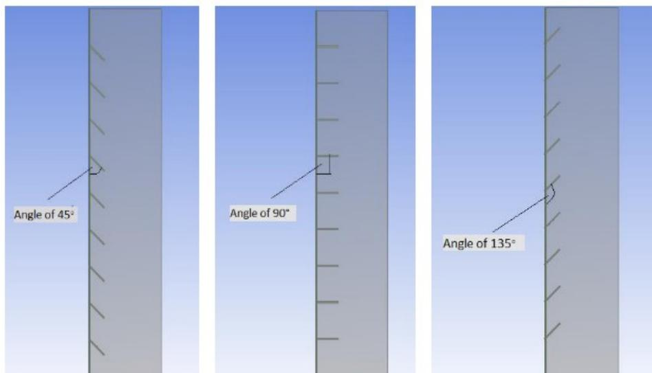
Figure 5. Inclination angles of the ribs for the studied case [39]
