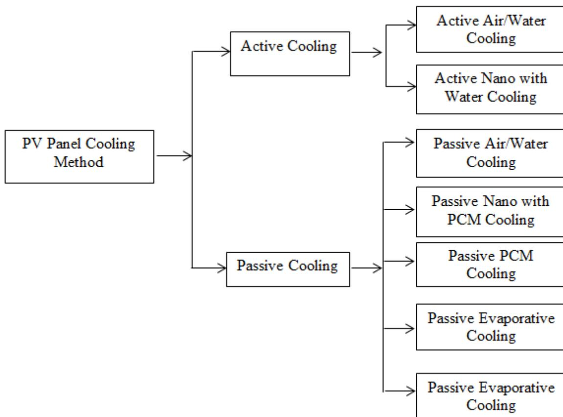
Figure 4. Classification of photovoltaic cooling techniques [1]
