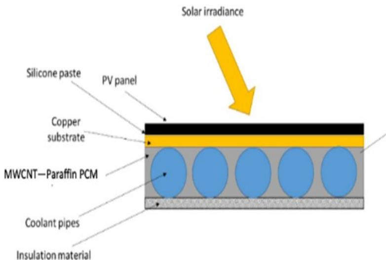
Figure 13. Mixture of PCM and nanoparticle cooling [102]
