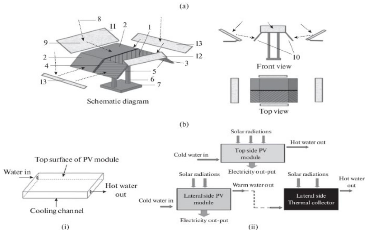
Figure 8. (a) Experimental setup and views. Legends: (1) glazing cover; (2) PV modules; (3) thermal collectors; (4) thermal separator; (5) cooling channel with glass wool insulation; (6) supporting columns; (7) base; (8) incoming solar radiation; (9) reflected radiation; (10) lateral surface; (11) south-facing mirror; (12) north-facing mirror; and (13) lateral side mirrors. (b) Mechanism of heat extraction from PV module. [63]
